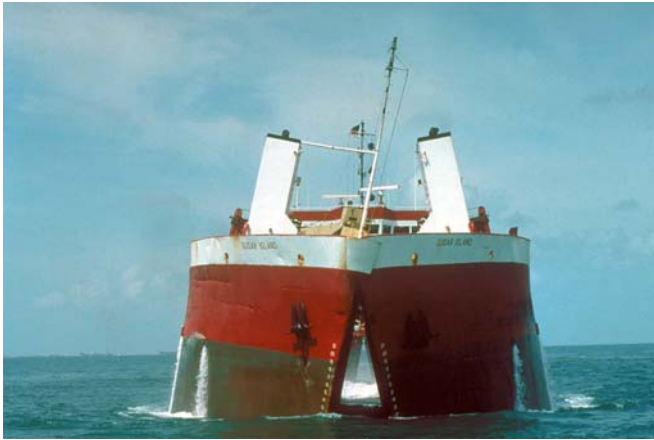
Figure 10-2. From the Manual, Industry Hopper Dredge SUGAR ISLAND splits its Hull in Gulf of Mexico near Galveston, Texas
